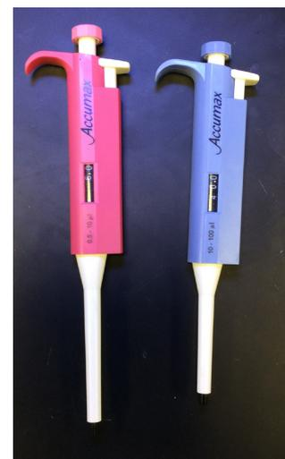
**Figure 2.6** A set of two digital micropipets. The pipet on the left delivers volumes between 0.5  $\mu\text{L}$  and 10  $\mu\text{L}$  and the pipet on the right delivers volumes between 10  $\mu\text{L}$  and 100  $\mu\text{L}$ .
