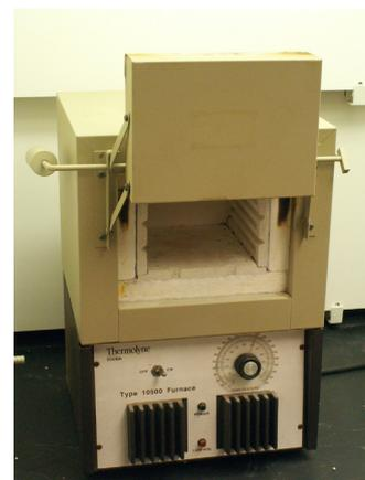
**Figure 2.10** Example of a muffle furnace.
