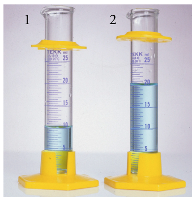
Figure 3.3 Two graduated cylinders, each containing 0.010 M \text{Cu}(\text{NO}_3)_2 . Although the cylinders contain the same concentration of \text{Cu}^{2+} , the cylinder on the left contains 1.0 \times 10^{-4} mol \text{Cu}^{2+} and the cylinder on the right contains 2.0 \times 10^{-4} mol \text{Cu}^{2+} .
